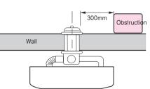
■ Flue fittings must be positioned away from flammable materials.
