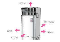
■ Do not allow curtains or other flammable materials to come into contact with the unit.
