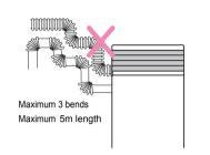
• Condensed water can form in the tube when extended. Make sure there are no low spots. Do not run the tube horizontally. If condensed water comes in to the heater, the water tray can overflow. Do not run flue more than 2m vertically.
