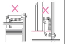
• The length of air inlet hose and the length of flue tube must be same.
