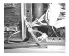
\* These condensing water heaters require a bracket for the control board:
