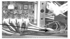
7) Run the other end of Communication Cable B through the cable access in the bottom of Unit 2's cabinet.
