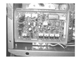
2) Connect the connector from Communication Cable A (18 inch, 450 mm cable) to socket No. 1 on Control Board.
