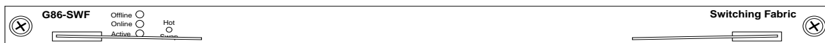
Figure 4-3 Location of offline LED and hot swap button on a switching fabric module
