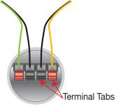
Depress the terminal tabs on the back of the RTS3000T. Insert speaker wires, black wires are negative (-) wires, color wires are positive (+) wires. Color of your wires may be different than shown here.
