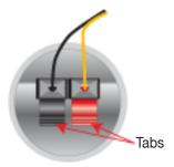
Depress the tabs on the back of the RTS2000T, insert speaker wires, black wires are negative(-) wires, color wires are positive(+) wires. Color of your wires may be different than shown here.
