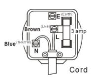
The wire coloured BLUE must be connected to the terminal marked N or coloured BLACK.
