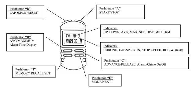
The indicators in this illustration will appear only when a particular mode or function is activated by pressing a pushbutton.
