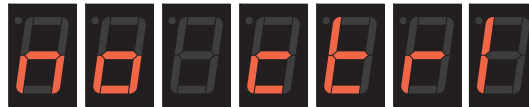
FIGURE 51. "No control" message will scroll when no valid radio signal is present
