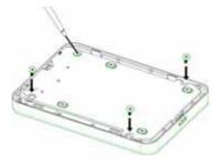
6 Replace the top cover and slide the lock switch to the right to lock the enclosure.
