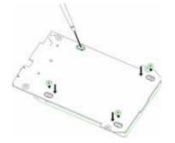
5 Place the printed circuit board/hard drive assembly into the enclosure with the hard drive face down, then secure it into the enclosure with the screws (4) you previously removed.
