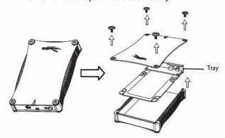
2 Place the hard drive into the tray, connecting the data connector to the corresponding connector on the printed circuit board, then secure the drive to the tray with four screws (provided).
