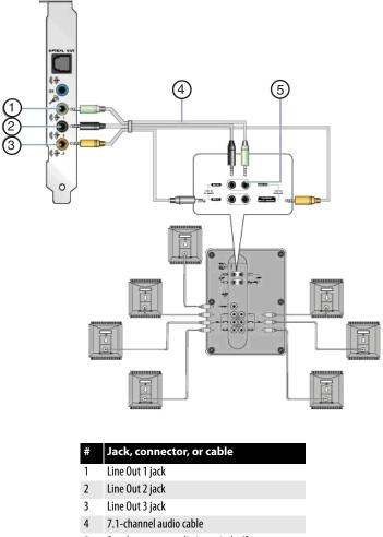
5 Speaker system audio input jacks (front, rear, side, and center/subwoofer)
