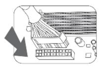
7 Connect the 8-pin (4+4) or 4-pin +12 V power connectors to your motherboard.
