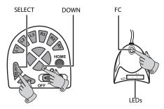
3 Press **FC** on the receiver. The LED on the receiver lights solid. This indicates the forced connection has been made.
