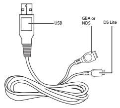
**3** Plug the DS Lite connector on the included USB cable into your DS Lite.
