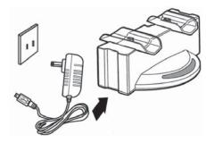
**3** Attach the Sony PS3 controllers to the charge station. The blue charging indicator on the charge dock lights up when the controller is connected.
