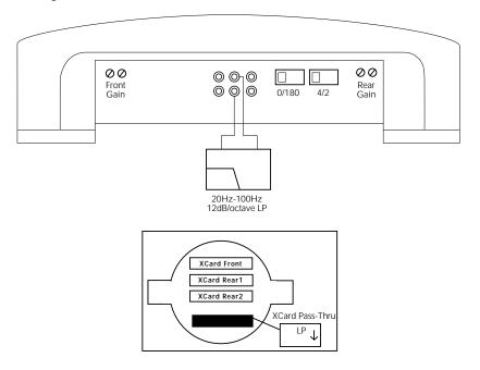
• Pass-Thru XCard set to High-Pass or Low-Pass
