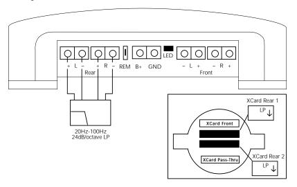
• Rear XCards 1 & 2 set identically to High-Pass or Low-Pass
