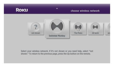
**NOTE:** The waves radiating from the center of the icon indicate the strength of the wireless network connection. A weak network connection may impact the quality of the video you receive with your player.
