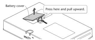
3 Install six AA alkaline batteries.
