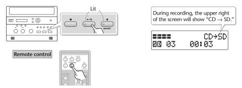
When CD playback stops at the end of the song, recording will also end automatically. If you want to stop recording in the middle of the song, press the [■ (Stop)] button. The recorded song will be added to the end of the SD memory card. If you want to listen to the song you recorded, press the [▶/II (Play)] button immediately after you stop recording.
