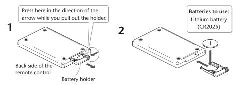
\* Use only the specified type (model no.CR2025) of lithium battery. Be sure to insert it as directed to ensure correct polarity.
