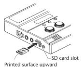
With the printed surface of the SD memory card facing upward, insert the card until it clicks into position.
