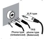
Both balanced and unbalanced connections are possible.
