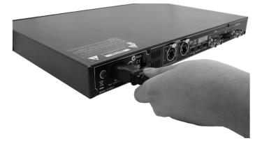
2. Secure the power cord in place with the cord hook.
