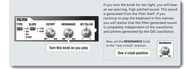
On a piano, its initial sound would include most of the harmonics that generates bright sound. Afterward, the sound would fade gradually, as a decrease in harmonics will result in a dull (dark) sound. To re-create this phenomenon, create a time-varied effect with the filter. In other words, the operation of turning the **[CUTOFF]** knob becomes automated as you play the keyboard.
