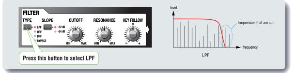
urn the **[CUTOFF]** knob as you play. Slowly turn it counter clockwise from all the way right (MAX) leftward to (MIN). The sound will gradually muffle during this process, and when it is turned left all the way, most of the sound becomes inaudible. This is due to the fact that most of the sound frequencies have been filtered out and rejected.
