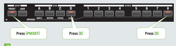
his patch is using the sawtooth wave of the OSC1 (oscillator 1). Play the keyboard, and hear the sound of this waveform. The sound at this stage is very simple and expressionless. To hear how the sound changes with each step, play the keyboard after each process.
