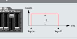
Move these **[A]**, **[D]**, **[S]**, and **[R]** sliders up and down, and listen to how it affects the sound. Afterward, to leave some lingering sound after releasing the hand, leave the **[R]** slider at the mid-high position.
