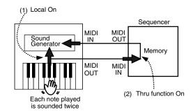
\* When a Roland MT series instrument is connected, it is not necessary to make the Local Off setting. The MT transmits a Local Off message when the power is turned on. If you turn on the power in the order of the HPi-7 → MT series, Local Off will be set automatically.
