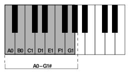
While V-LINK is switched on, no sound is produced when you press any of the twelve keys at the left end of the keyboard.
