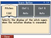
Detailed settings for functions are made in a screen similar to this. The currently selected item will be highlighted, and you can use the [+] [-] buttons to edit the value. An explanation of the selected item is shown below the item. For some items, an explanation of the values will also be displayed.
