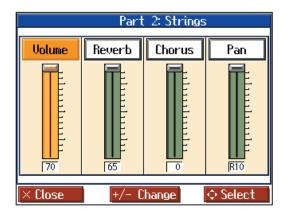
**2** Press the [ ◀ ] or [ ▶ ] button to select the parameter, then change the value with the [+] or [-] buttons.
