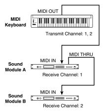
When used as a sound module, the TD-6V can receive on up to six of the sixteen MIDI channels (16 channels in GM mode). Sound modules like the TD-6V which can receive multiple MIDI channels simultaneously to play different sounds on each channel are called "multi-timbral sound modules."
