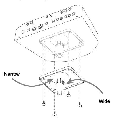
Attach the TD-6V and stand holder to the drum stand (such as the
