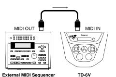
2. Send the settings data from the external sequencer to the TD-6V.
