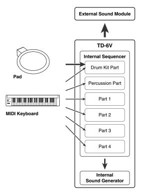
For playback, the performance data that has been recorded to the sequencer is sent to the sound module, which produces the sound. The data for each of the sequencer's parts causes the corresponding part in the internal sound module to be played. When performance data is recorded, the performance data from pads and MIDI keyboards is sent to the sequencer; the data recorded here is then sent to the sound module for playback.
