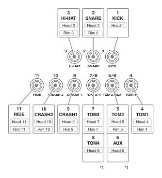
\*1: By using an optional cable (the PCS-31) or standard insert cable, you can use two pads to a single trigger input jack. In this case, the rim sounds of "Trigger Input 5 (TOM2)" and "Trigger Input 7 (TOM 3)" become unavailable. For more on how to make the necessary connections, refer to p. 21.
