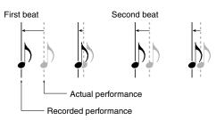
This is usually set to the shortest note appearing in the phrase to be recorded. When set to "OFF," the pattern is then recorded with the timing used in performance.
