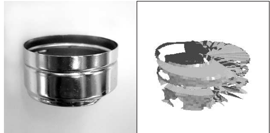
Plated object Rotary scanning Pitch: 1.0 mm x 3 degrees
