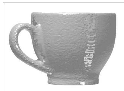
Plane scanning (four scanning surfaces)
