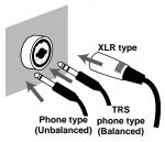
Both balanced and unbalanced connections are possible.
