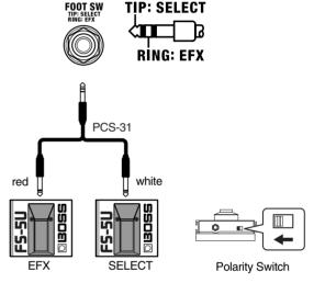
\* When you connect only one footswitch by mono cable, you can only use it to switch channels (JC CLEAN/LEAD).
