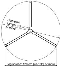
When deciding on a stand to use with the KC-60, make sure to pick one that is capable of supporting its weight.  Before use, adjust the speaker stand to a height of 165 cm (65") or less and a leg spread of 120 cm (47-1/4") or more, as shown in the figure below.
