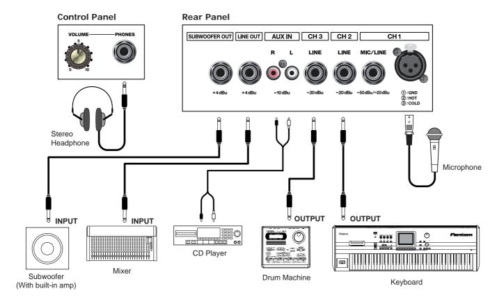
Here is an example of a setup that makes full use of the KC-60's mixer and monitor functions.
