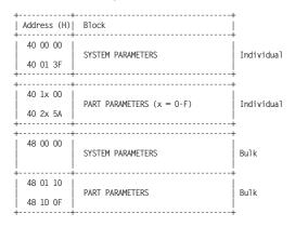
There are two ways in which GS data is transmitted: Individual Parameter Transmission in which individual parameters are transmitted one by one, and Bulk Dump Transmission in which a large amount of data is transmitted at once.
