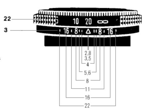
**20** feet (or **2** and **6** at meter scale) are marked in red on the distance ring **22**. At a medium aperture (f/8 to f/11) these settings provide extended focusing ranges:
