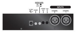
INPUTS: 1 - 2: XLR balanced inputs for connection to any standard dynamic or condenser microphone. The input circuitry has a very wide input range and can accommodate almost any (mic to line) level signal.
