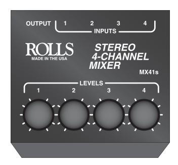
PLEASE NOTE: The MX41s is to be operated with all mono inputs, or all stereo inputs only. Using combinations of stereo and mono will degrade the unit's performance.
