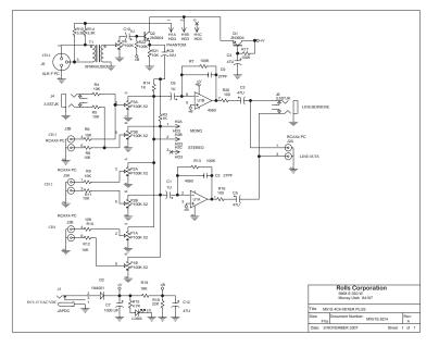
signals to a mono output. ... anywhere you need to mix up to four line
