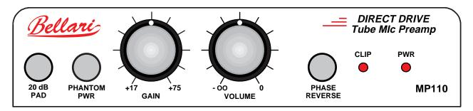
The MP110 provides clear sonic quality and performance for the working musician, studio operator or anyone who needs a preamp with the warm, smooth, analog sound. The unit uses a premium 7025 tube in a unique configuration to give smooth controllable gain. The unit has both XLR and 1/4" inputs and outputs with a 20 dB Pad and a Phase Reversal switches to adapt to any performing or studio situation.
