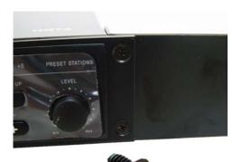
Use the flat head screws to attach the front of the unit to the rack ears. After the flat head screws are in go back as described above and fully tighten the side round head screws. NOTE: YOU ARE ATTACHING A METAL BRACKET TO PLASTIC. DO NOT OVER TIGHTEN THE SCREWS AS THEY WILL EASILY BREAK THE PLASTIC FRONT OF THE UNIT.
