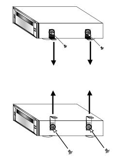
Finally, attach the mounting brackets to the mounting surface in a safe and secure fashion.
