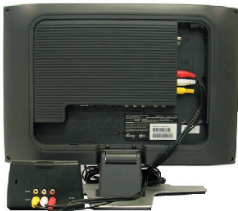
2. Typical connection DVR output to TV input
