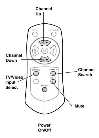
NOTE: Some buttons on the AC3105 remote control do not operate with the AC3105 - they are for other applications using optional equipment. All operating buttons are highlighted in the diagram above.
