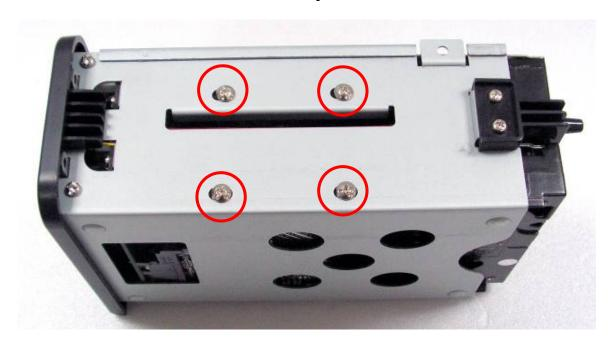
**STEP5:** Push the tray into the aluminum case. Screw the rear panel and enclosure together.
