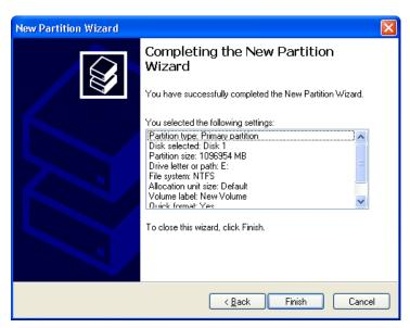
**STEP7:** When new partition is completed, the external HDD will be recognized as a "New Volume".
