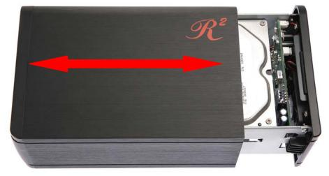
**STEP2:** Place the first HDD into the tray. Push the HDD to connect the SATA connector.
