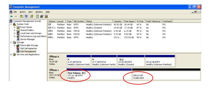
Right-click the red-squared block and select "Delete Partition". Delete both HDDs' partition then start to format two HDD into one.
