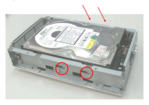
**STEP5:** Reassemble two side plates back to the enclosure and fix the screws.
