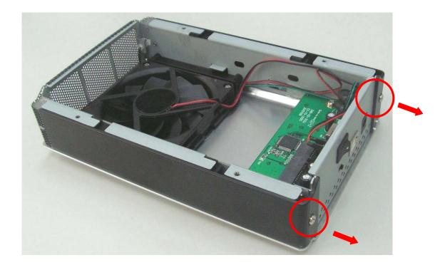
**STEP3:** Place HDD into the enclosure properly. Connect HDD to SATA connector.
