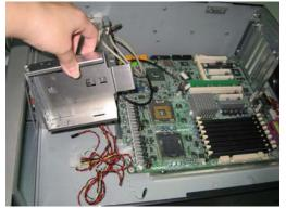
• Install 3 x 3.5" device into 3.5 drive bay and secure it
