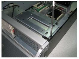
• Remove drive bracket from chassis.
