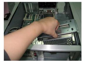
• Install 3 x 5.25" device into front 5.25" drive bay
