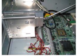
Drive bracket being removed
