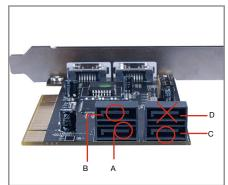
Note: There are six SATA ports in Serial ATA 4-Channel RAID adapter. We named these ports character A through F. Ports A to D are internal SATA ports and E & F are external SATA ports. By changing the jumper setting on the Serial ATA 4-Channel RAID adapter that allows you to select between external and internal ports to use. By default, Port A, B, C and D are working.
