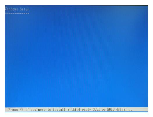
e. Keep the floppy in floppy drive and follow the installation. Press "S" when the screen shows as the following picture.
