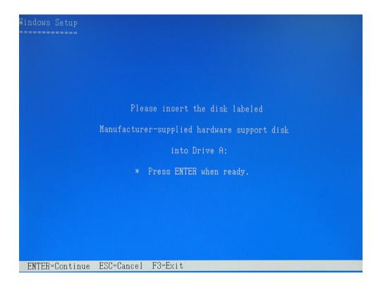
The installation of RC-209 by floppy drive will be completed and the system will detect the HD which now plug on the card.
