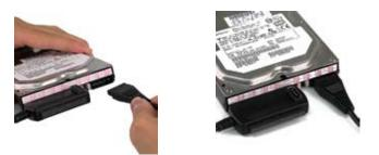
Plug the power adapter to power source and turn on the power . (Please make sure the voltage is between 100~240V)
