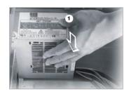
1.Place the power supply into the case
