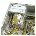
4. Hook the hole of one-side clip onto the lug of Retention frame, and hook the hole of another-side clip onto the lug of Retention frame. Press down the clip on the hooks and fasten the levers properly by using a finger and a phillips screwdriver (+) onto a hole together.
