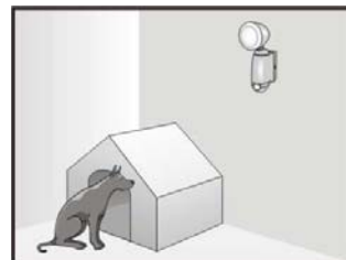
*Avoid installation in places where there would be eternal movement with animals.
