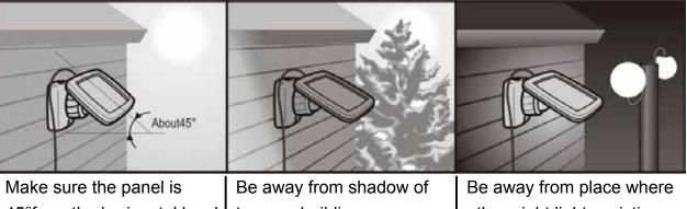
45° from the horizontal level. This angle can be adjusted.
