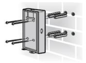
3.slip the PIR Solar Spotlight body up to 4.adjust the angle of light head & PIR down until the hasp inside is connected, fix sensor the body with screws.
