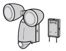
2.drill 4 holes on the wall based on the four tubes in the battery back cover, insert the bulged tubes in the holes, and fix the battery back cover with screws.
