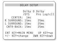
This menu, which is reached from the MAIN menu, allows you to set the delay for individual speakers. This ensures that the sound from each speaker arrives simultaneously at the listening position, even when the speakers are not all placed at equal distances from the listener.
