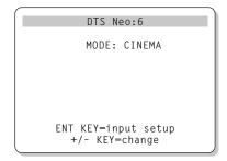
When Dolby Pro Logic II or DTS Neo:6 is selected as the default surround mode on the INPUT SETUP menu (see previous section), there are additional option settings and parameters available to optimize the surround decoding for various types of recordings, music or movie soundtracks.
