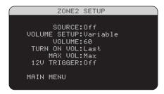
The ZONE 2 SETUP menu provides settings and configuration options related to the operation of Zone 2. This menu is reached by highlighting the ZONE 2 line on the MAIN menu and pressing ENTER.
