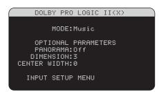
When Dolby Pro Logic II (x) is selected as the default surround mode on the INPUT SETUP menu, there are additional settings and parameters to optimize the surround decoding for music or movie soundtracks. Dolby Pro Logic II uses matrix decoding algorithms to derive a center channel and surround channels from 2-channel source material.
