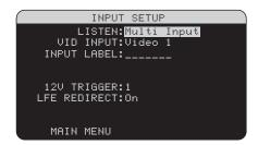
When the MULTI INPUT source is selected on the INPUT SETUP menu, the available options change to reflect the fact that these inputs are direct analog inputs and bypass the RSX-1056's digital processing. The INPUT, CINEMA EQ, and DEFAULT MODE options are not available since these are all digitally implemented features.
