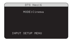
When DTS Neo:6 is selected as the default surround mode on the INPUT SETUP menu, there are additional option settings and parameters available to optimize the surround decoding for various types of recordings, music or movie soundtracks. DTS Neo:6 uses matrix decoding algorithms to derive a center channel and surround channels from 2-channel source material.
