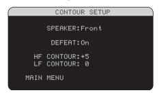
The CONTOUR SETUP menu allows digital adjustment of the bass and treble response of each group of speakers in the system. For example, if your center channel speaker sounds too bright, you could roll off the extreme high frequencies.
