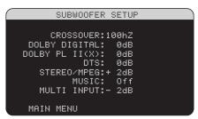
The SUBWOOFER SETUP menu allows selection of the master subwoofer crossover frequency and independent adjustment of subwoofer level for each surround mode.
